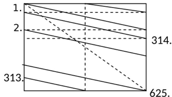
Figure: TV scanning pattern (Left), Interlaced scanning (Right)
